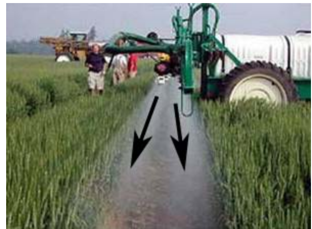
Figure 4—Twin Jet Nozzles
